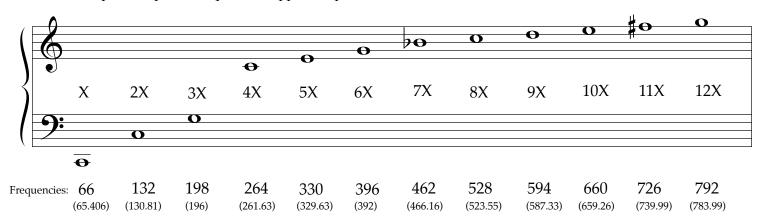
The "Major Scale" can be derived from the 4th 5th and 6th partials of three harmonic series: the one on "X," in this case "C," the one on "3X/2" ("G") and "2X/3" ("F"), resulting in "Just Intonation."
